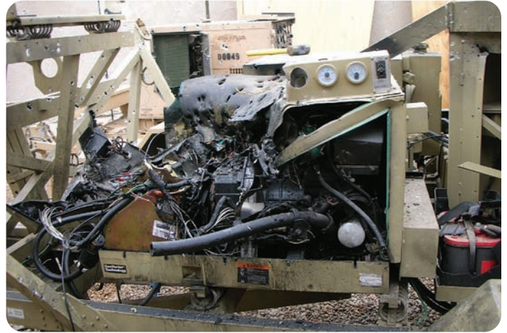
In the second incident in December 2006, this STT received a direct mortar hit.
